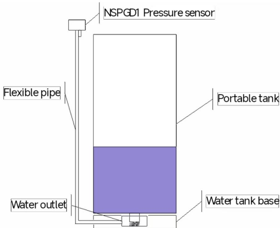
Figure 6.1 Portable tank structure
