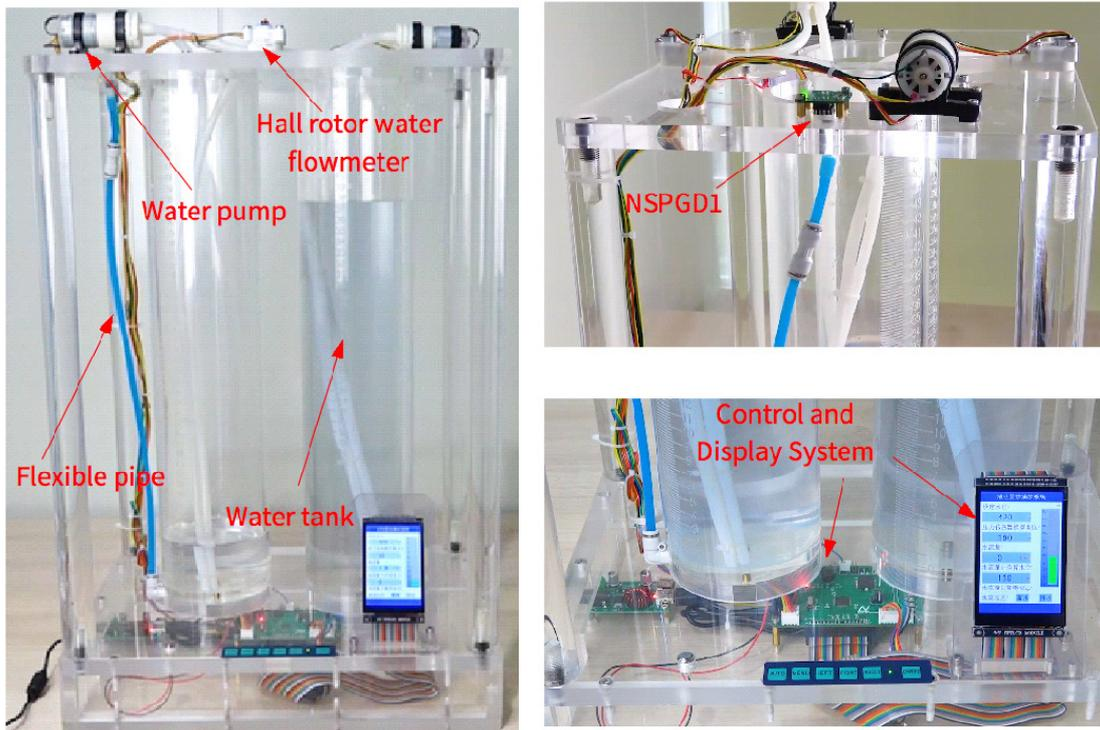
Figure 8.1 Liquid level test DEMO
