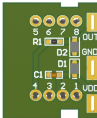
Figure 5.1 Water level sensor PCB layout
