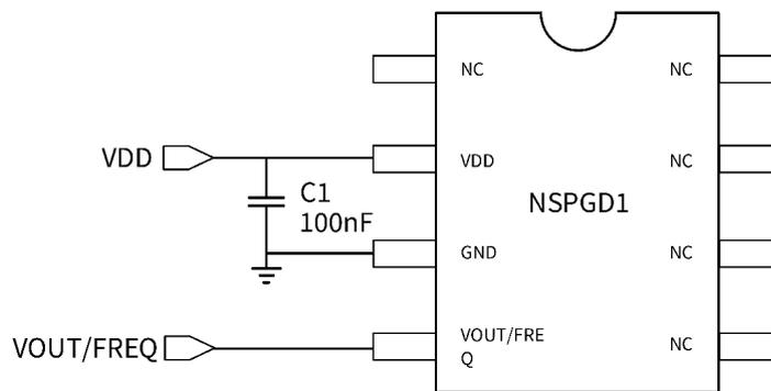
Figure 4.1 Analog/ Frequency Output Application Circuit
