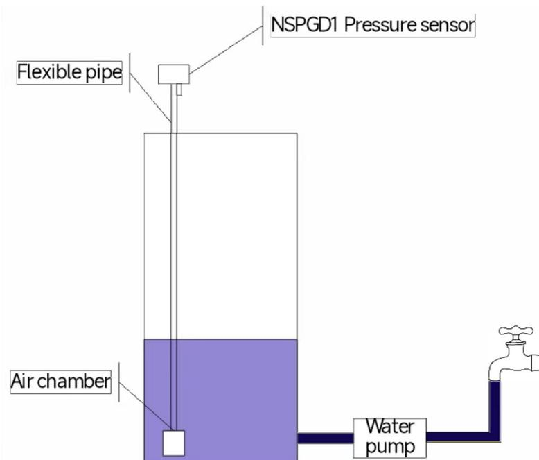
Figure 6.3 Independent air chamber water tank structure
