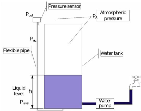
Figure 2.1 Hydrostatic pressure
