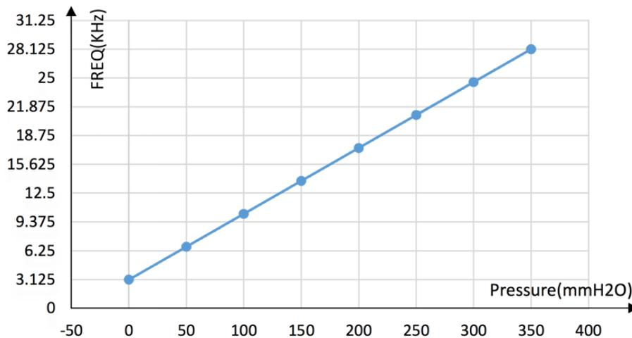
Figure 3.2 Typical frequency output curve
