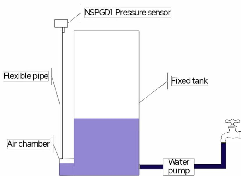
Figure 6.2 Air chamber integrated water tank structure
