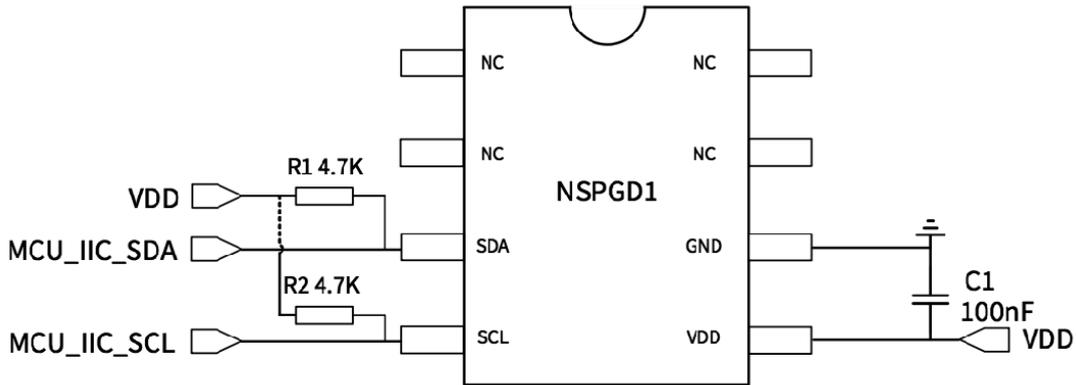
Figure 4.3 I<sup>2</sup>C Output Application Circuit
