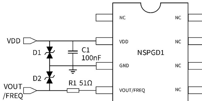
Figure 4.2 Analog/ Frequency Output Protection Circuit
