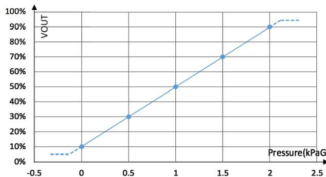
Figure 3.1 Typical analog output curve
